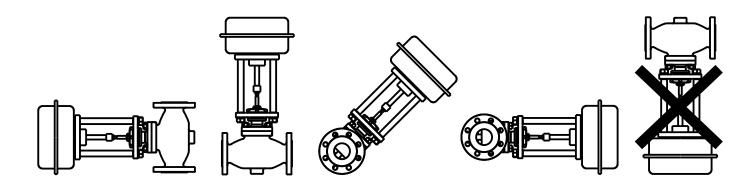
Pic. 3: Installation position for valves with electro- or pneumatic actuators
