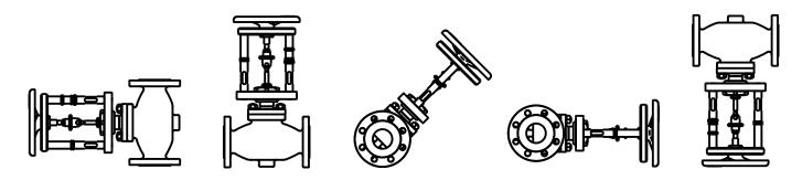
Pic. 4: Installation position for valves with hand wheel
