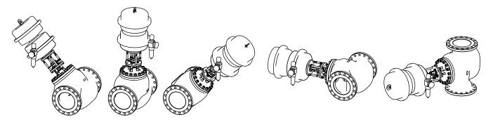
Pic. 7: Examples of filter/regulator position
