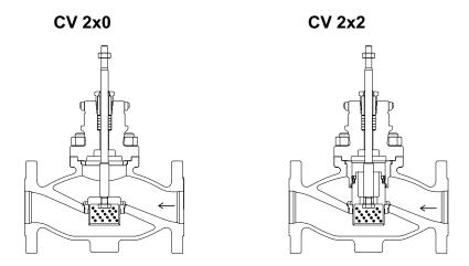
Pic.2: Flow direction for valve with perforated plug CV 2xx xxx xxxx **D**x xx/xxx-xxx (Char. **D**; **Z**; **Q**)
