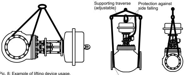
Pic. 8: Example of lifting device usage.
