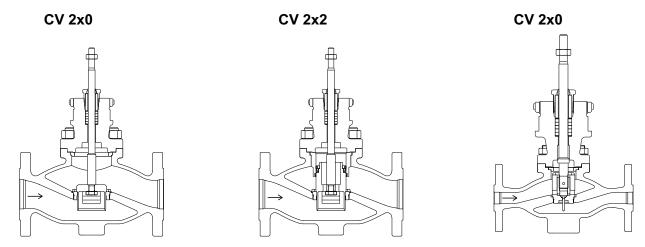
Pic.1: Flow direction for two-way valve with V-ported or contour plug CV2xx xxxx Lx xx/xxx-xxx Ex (Char. L; R; P; S; U)
