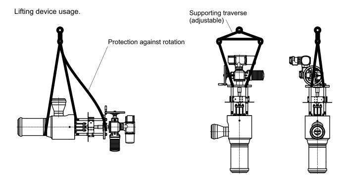
It is necessary to make sure the valve can not be damaged during transport. **Special attention shall be paid to** the valve stem, stroke indicator and outside accessories fixed to the actuator. Never lift the valve by the lifting device fixed on the actuator only!
