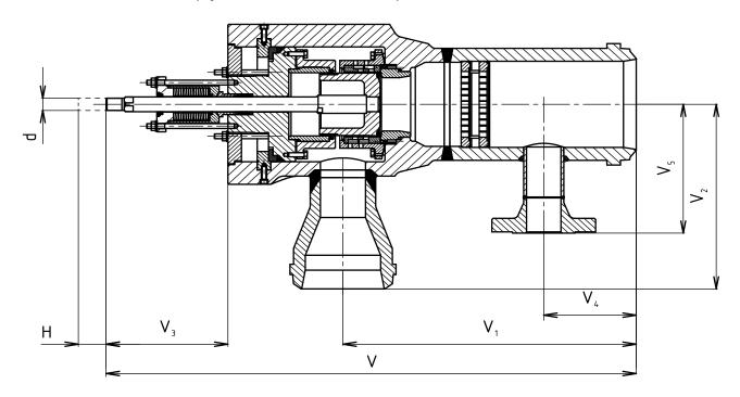
Steam-conditioning station RS 902 /Rx - connection for CHR ( (injection perpendicular to the axis of outlet)
