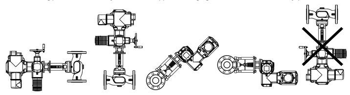
Pic. 3: Installation position for valves with electro actuators
