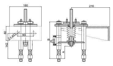
Pic.4: Fixing bracket for DN15 to 25 valves.
