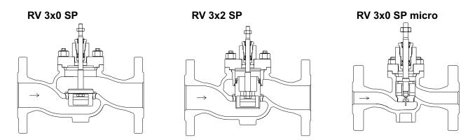
Pic.1: Flow direction for two-way valve with V-ported or contour plug RV 3xx xxx xxxx Lx xx/xxx-xxx SP (Char. L; R; P; S; U)
