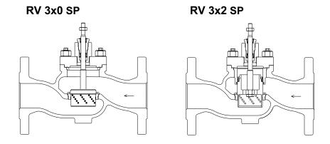
Pic.2: Flow direction for valve with perforated plug RV 3xx xxx xxxx **D**x xx/xxx-xxx SP (Char. **D**; **Z**; **Q**)
