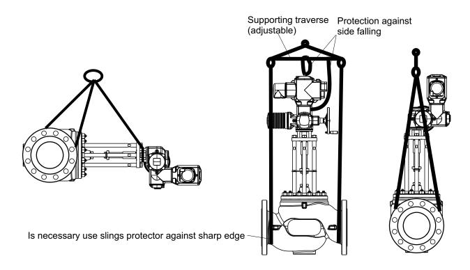
Pic. 8: Example of lifting device usage.
