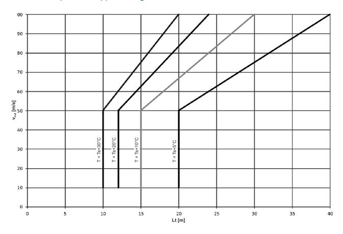
Steam cooling near the saturation point is very complicated because the steam and water multiphase flow appears here and a lot of injected water does not vaporize. Droplets of water negatively affect the accuracy of temperature measurement which may cause flooding or conversely overheating of the steam pipeline. In the case
